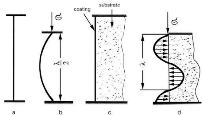
**Fig. 3.** Buckling instability for an anisodiametric body in a free state (a, b) and on a soft substratum (c, d).
