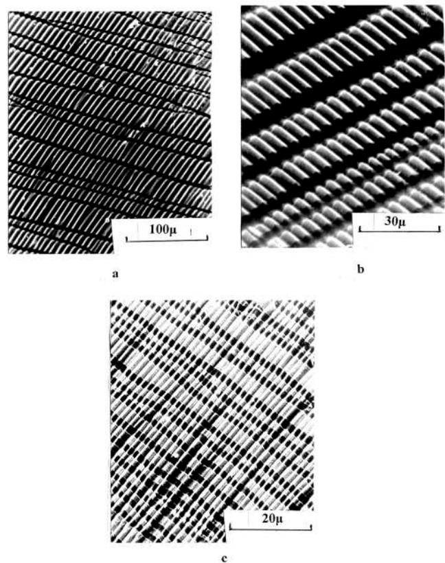
**Fig. 1.** SEM image of the NR sample with thin (15 nm) gold coating after its deformation at room temperature to tensile strain 50% (a); PVC sample with a thin (21 nm) platinum coating after its deformation at 90 °C to a tensile strain of 20% with a strain rate of 10 mm/min (b); and PET sample with a thin (15 nm) platinum coating after its deformation at 90 °C to a tensile strain of 100% with a strain rate of 1 mm/min (c).
