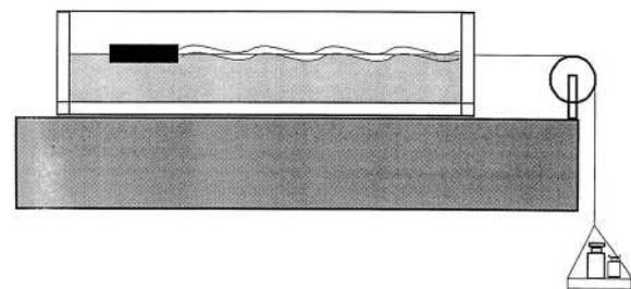
**Fig. 4.** Schematic representation of the equipment used for modeling of folding by Ramberg and Stephansson [18].
