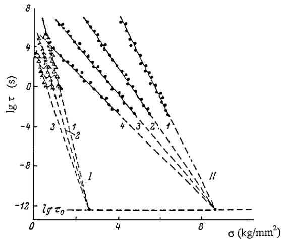
**Fig. 10.** Durability (lifetime) *vs.* tensile stress for (I) rock salt at 1) 400, 2) 500, and 3) 600 °C and (II) semicrystalline aluminum at 1) 18, 2) 100, 3) 200, and 4) 300 °C [18].
