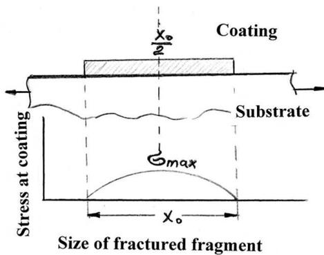
**Fig. 5.** Schematic drawing of a coating fragment adhered to a polymer substrate. The  $X$ -axis is chosen so that in the center of the fragment  $x = 0$ .
