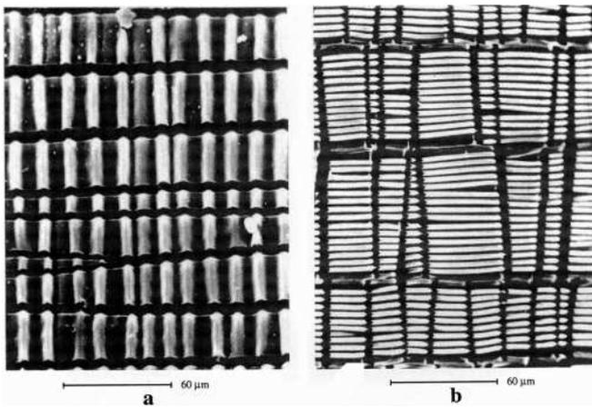
**Fig. 2.** SEM images of rubber samples coated with a thin (15 nm) platinum layer: (a) deformation is carried out for the Pt-coated sample to 50%; (b) initial rubber sample is drawn to a strain of 100%, the as-drawn sample was coated with Pt layer and allowed to shrink and recover its initial size. The axis of extension is vertical.
