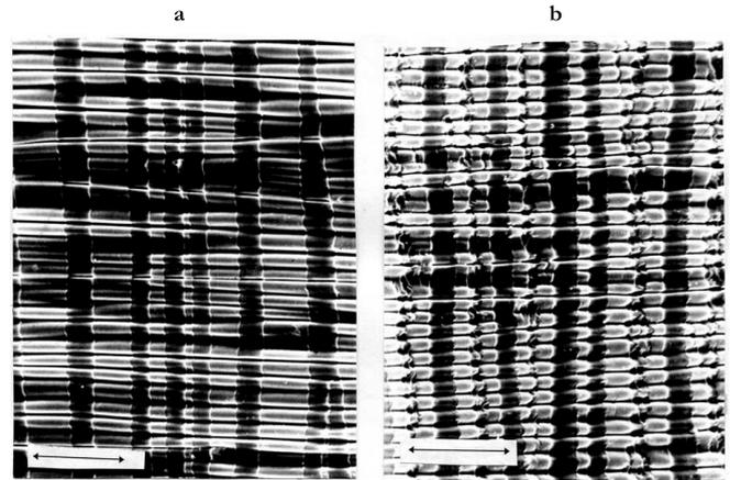
**Fig. 6.** (a) SEM micrograph of Pt/PET, elongated to 100% strain at a temperature of 100 °C. (b) Pt/PET elongated to a strain of 50% at 100 °C, and after that, elongated to a total strain of 100% at 85 °C. The cracks in the midlines of the fragment bands reveal the mechanism of fragmentation.
